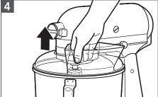
Lift the front of the pouring shield clear of the bowl rim and pull forward. Remove attachment and bowl.
